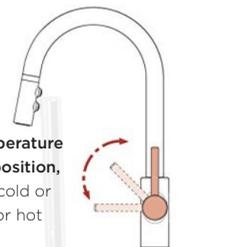
Adjust temperature by handle position, upright for cold or pull down for hot water.
