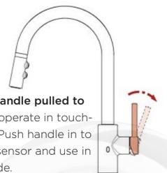
Leave the handle pulled to the side to operate in touch-free mode. Push handle in to deactivate sensor and use in manual mode.
